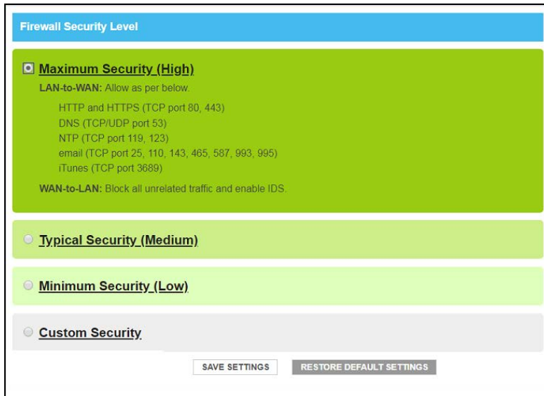
Figure 37: Firewall IPv4 high security level screen
